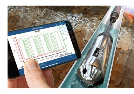
Onset's HOBO MX2001 is the industry's first water level data logger designed for convenient wireless setup and download from mobile devices via Bluetooth Low Energy (BLE) technology. The logger dramatically simplifies and lowers the cost of field data collection by providing wireless access to high-accuracy water level and temperature measurements right from a mobile phone or tablet.
