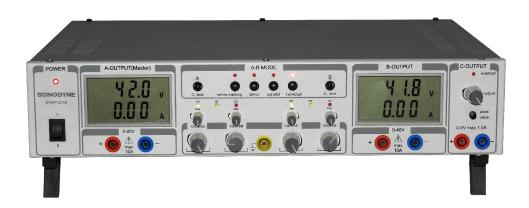
SVSP 2410 is a high quality triple output variable DC power supply. On the power supply's two main outputs, voltage and current can be controlled in the range of 0.1 - 40Vdc (0 - 10A) using separate knobs for fine and course adjustment and 0 - 6Vdc (max 1.5A) on the SVSP 2410's third output.
