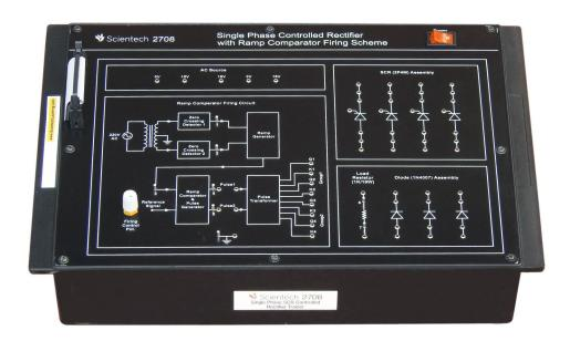
Scientech 2708 is a platform which helps Students to understand the various concepts of Ramp comparator firing scheme for Single phase controlled rectifier. 2708 is also useful for Students to understand the various rectifier configurations like half wave, full wave, bridge, symmetrical & asymmetrical configurations. This platform is provided with the built in AC & DC power supplies, sockets for making different interconnections in the circuit and exhaustive learning material.
