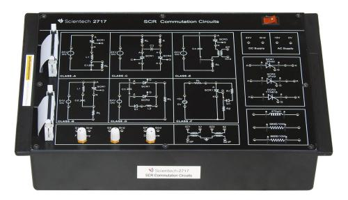
**Scientech 2717** is a platform which is very useful for Students to understand the concept of various thyristor commutation techniques for SCR. Platform is provided with various. Commutation circuits like Class A, Class B, Class C, Class D, Class E & Class F commutation. This platform is provided with Inbuilt AC/DC power supplies & exhaustive learning material are provided.
