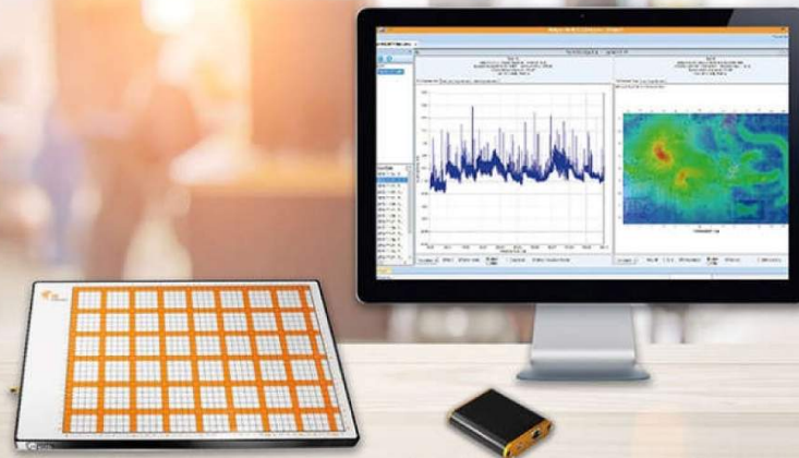
High speed real-time EMC/EMI Diagnostic tool
