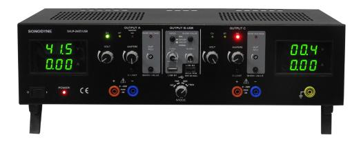
Linear Bench Power Supply unit eliminates voltage harmonics across the entire range of electrical loads and features separate USB ports for both R&D/QA and equipment charging. The device is suitable for any situation that involves pushing SMPS units to the limit. The SVLP-USB is robust and comes with short circuit and over voltage protection, and a thermal cutoff.
