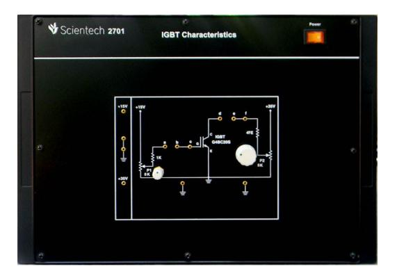
**Scientech 2701** is a platform which is very useful for Students to understand the VI characteristics of IGBT. 2701 is provided with in built power supply and exhaustive learning material.
