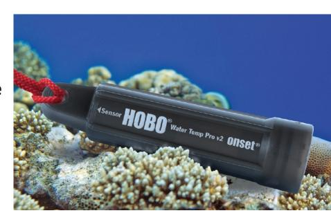
The HOBO Water Temp Pro v2 data logger features 12-bit resolution and a precision sensor for ±0.2°C accuracy over a wide temperature range. Designed with a durable streamlined case for extended deployment in fresh or salt water, the Water Temp Pro v2 is equipped with an Optic USB interface for data offload in the field, even when the data logger is wet.
