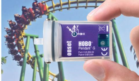
Measure 3-dimensional motion, such as sports activity or medical therapy compliance, with the HOBO Pendant G data logger. With this logger, users can measure acceleration and angular displacement in 1, 2 or 3 axes. Use this data to monitor activity and improve performance.
