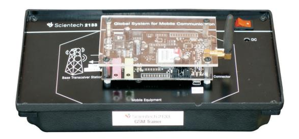
Scientech 2133 Global System for Mobile Communication platform is a modem or mobile equipment for transmission of voice and data calls as well as SMS (Short Message Service) in GSM Network.
