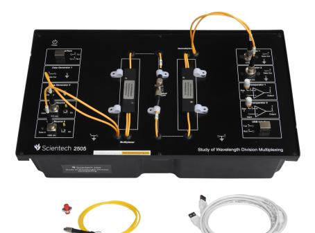
**Scientech 2505 Study of Wavelength Division Multiplexing** is designed for understanding WDM technique and Chromatic Dispersion measurement.
