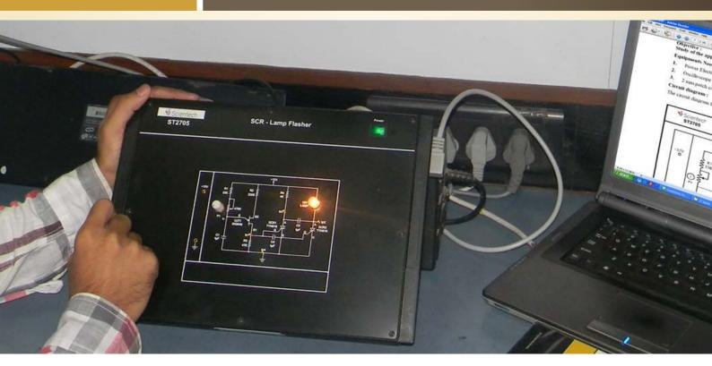
Scientech 2705 is a platform which is very useful for Students to understand the low voltage application of the SCR in lamp flashing. 2705 is provided with the built in power supplies, sockets for making different interconnections in the circuit, and exhaustive learning material.
