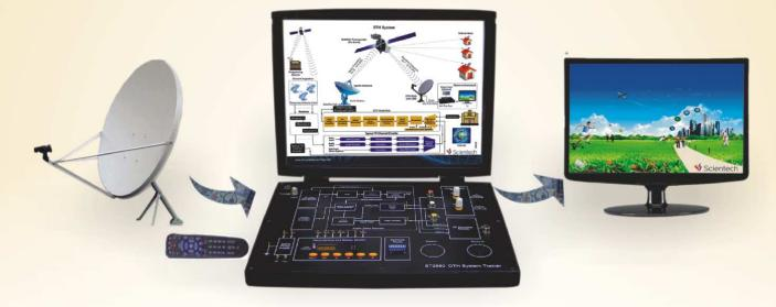
Scientech TechBook 2664 DTH Receiver System is a versatile platform useful for students to learn the concept of DTH and its troubleshooting. Scientech 2664 is housed in an elegant cabinet with proper block diagram on the mimic. 2664 is provided with fault creating and troubleshooting facility to understand the working of DTH.
