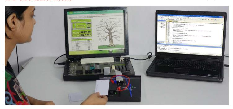
RFID Card Reader Module MC20RFID is an extension module for Nvis Microcontroller development platforms. The module has been designed for students and practicing engineers to gain invaluable practical experience on the principle and applications of microcontroller & RFID card reader. The objective is to have a clear understanding of how RFID card reader is interfaced and controlled with microcontroller.
