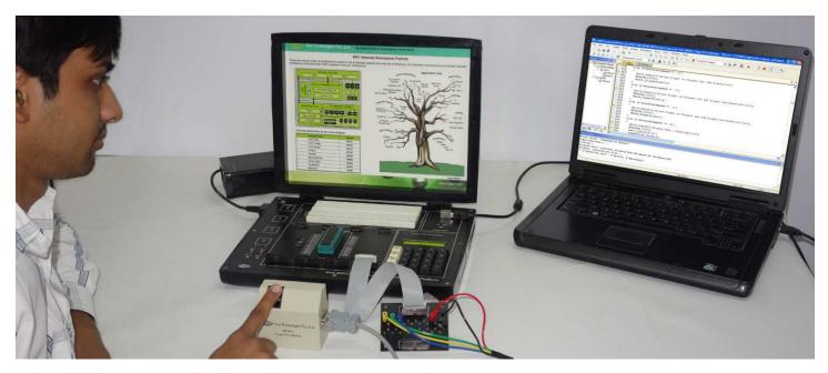
**Finger Print Module MC20FP** is an extension module for Nvis Microcontroller development platforms. The module has been designed for students and practicing engineers to gain invaluable practical experience on the principle and applications of microcontroller & Finger print module. The objective is to have a clear understanding of how Finger print module is interfaced and controlled with microcontroller.
