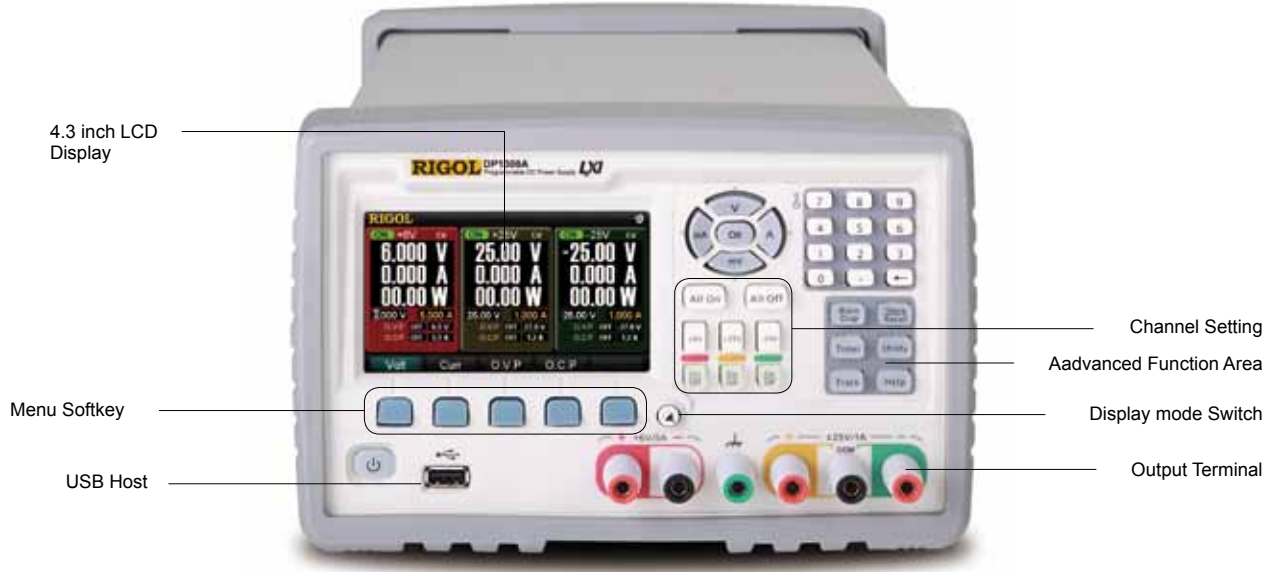
Product Dimension: Width×Height×Depth=235 mm×155 mm×384 mm Weight: 8.5 kg
